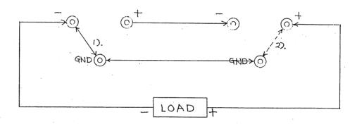
GND terminal shall be connected as follows.
