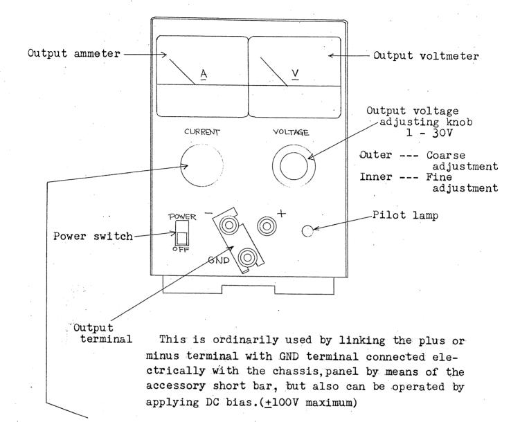
Current limiting knob This knob enables to limit output current in the range of O.lA ~ O.5A, within which this model can be used as a constant-current power supply.
